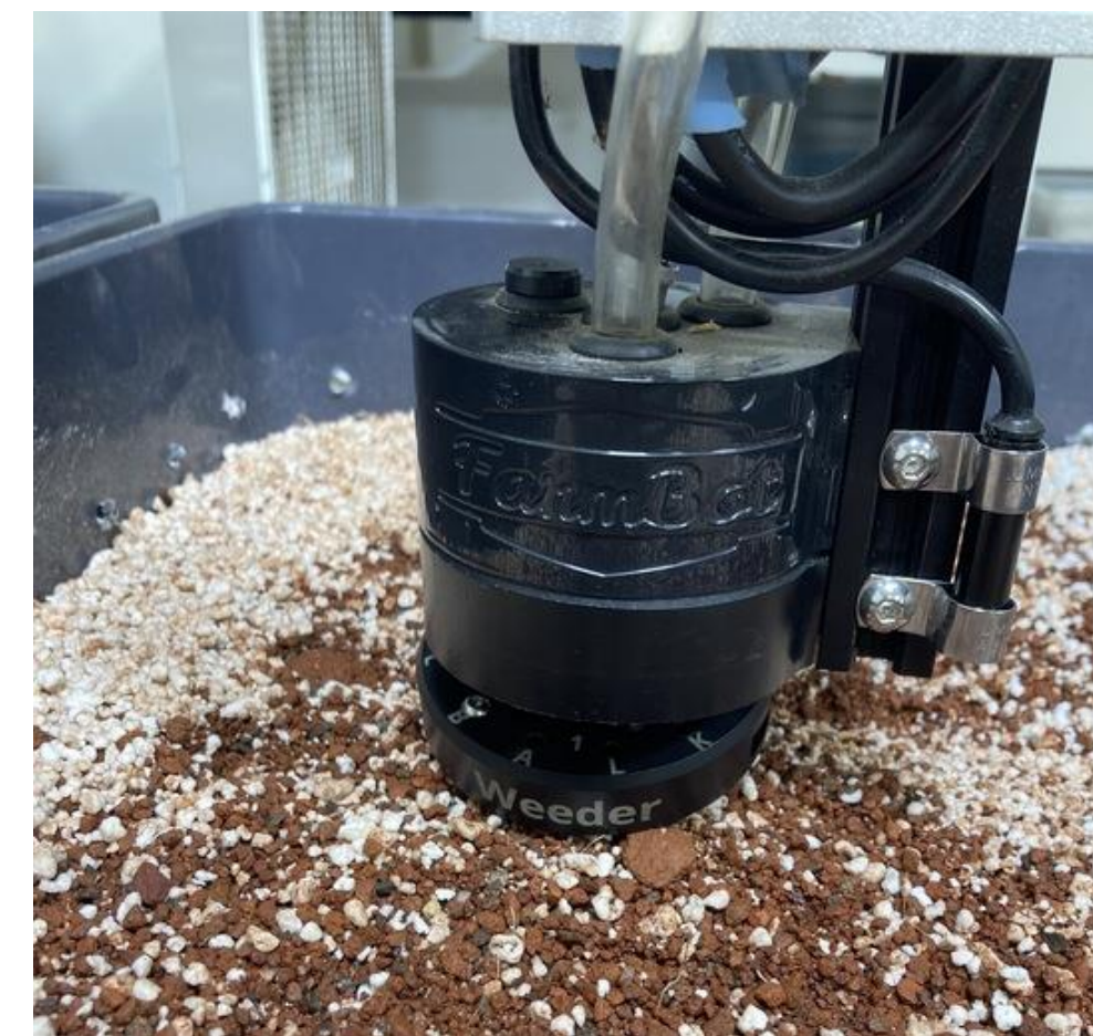
Figure 2: Weeder tool falling off the UTM due to unsifted regolith compaction, post watering.
