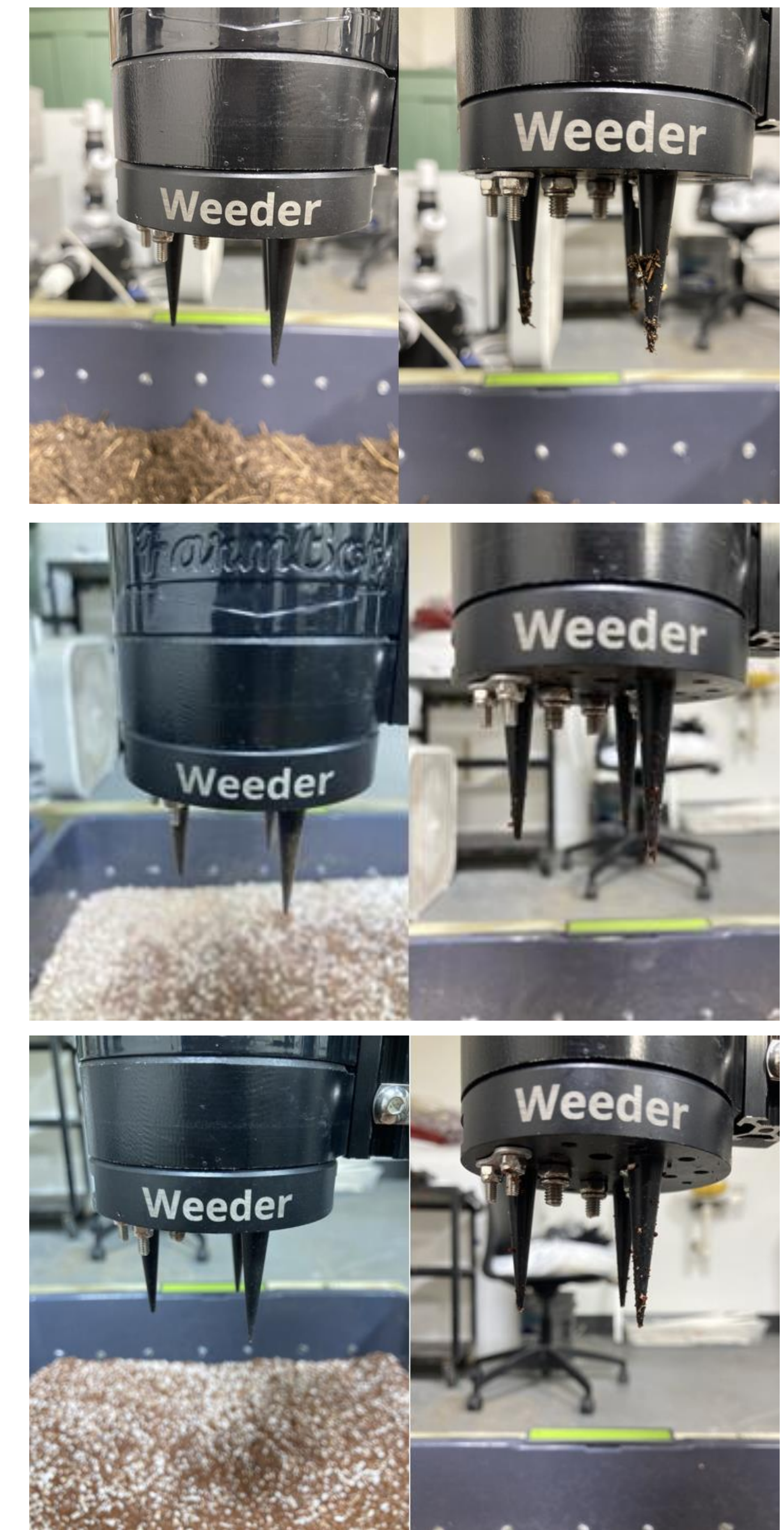
Figure 3: Visual observations of soil/regolith accumulation on the weeder tool, before and after watering substrate.
